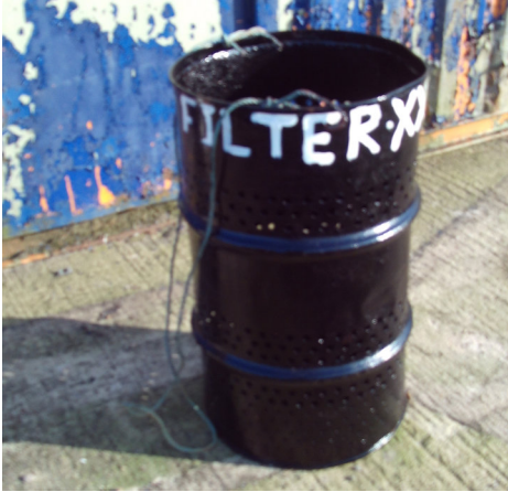
XXL pump filter. The local Steel Band were not best pleased
